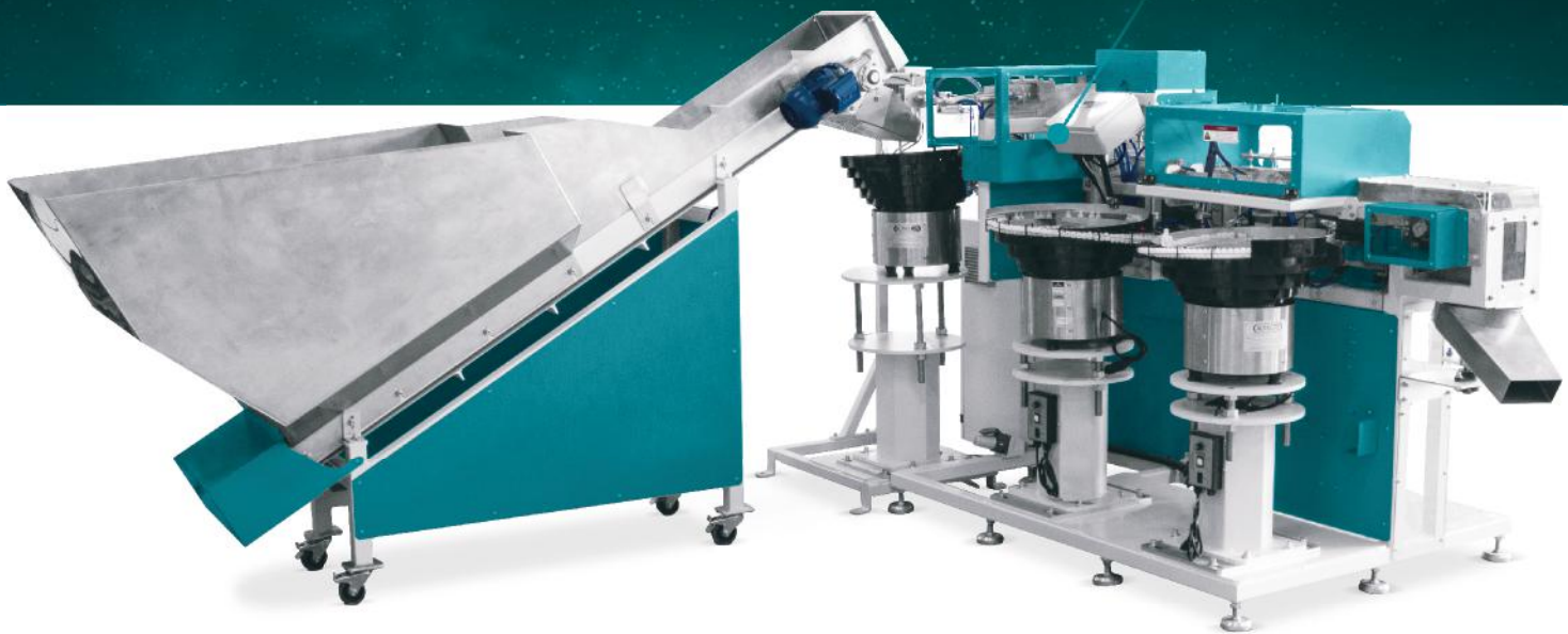
Test tube capper machine It delivers up to 120 sets (cap + tube) per minute
